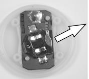
4. Replace the top and the gasket on the case. It will fit securely only one way—the sensor dome is on the side opposite the power button. Tighten the four screws.
